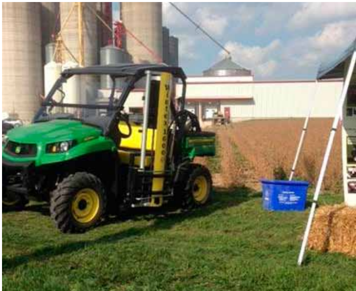
Soil sampling equipment used in the Medway Creek Priority Subwatershed study.
