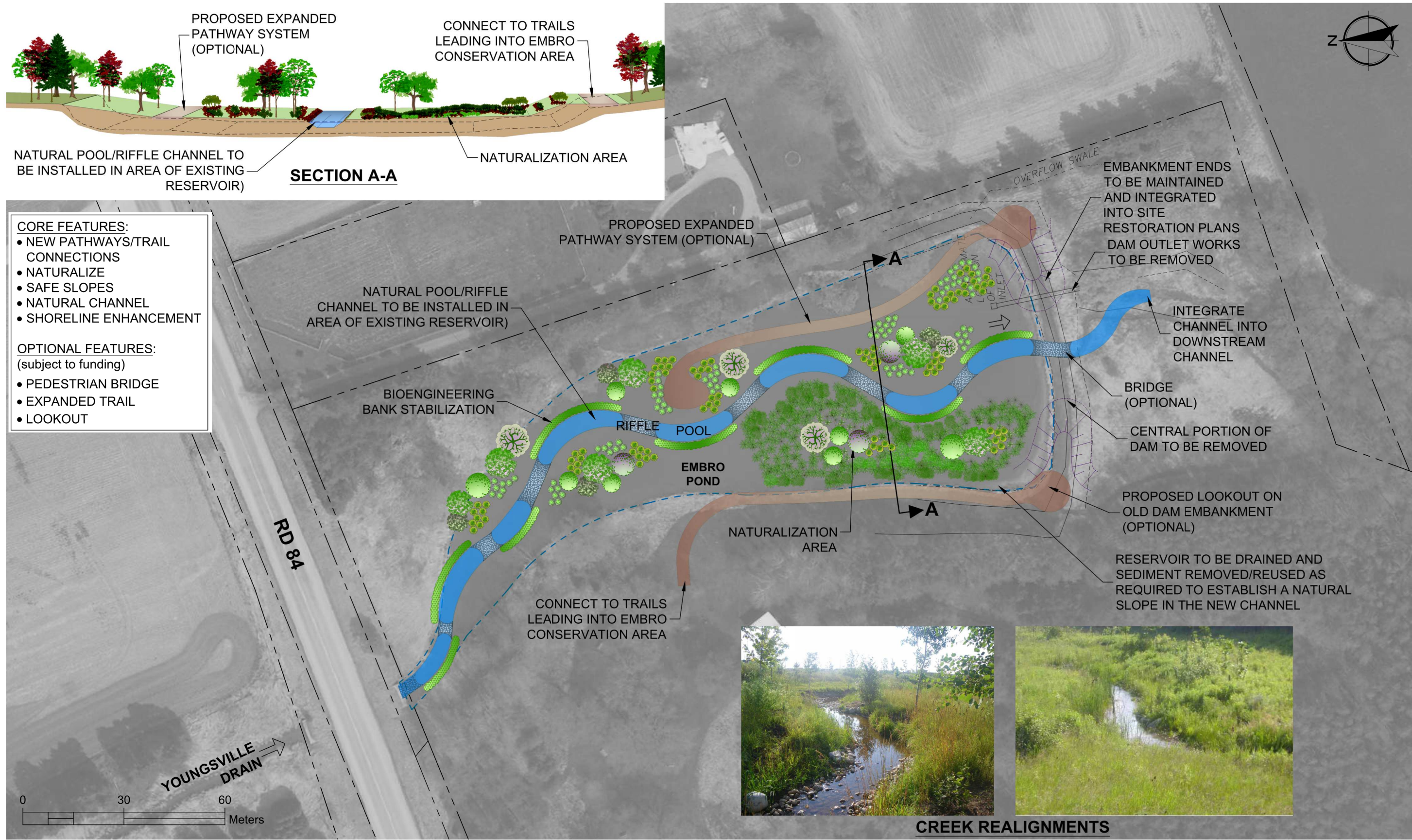
Figure 23 Alternative 3: Remove Dam and Construct Natural Channel
