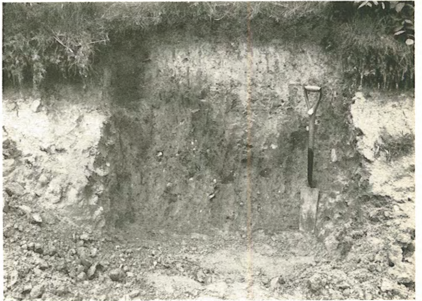
A cut to show the profile of Guelph loam. Under the dark loam of the topsoil is a light gray level. The reddish brown subsoil is beside the shaft of the spade.
