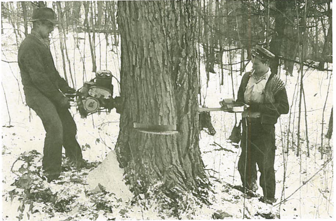
Professional power saw loggers can make up to 10,000 board feet of hardwood logs (Doyle Rule) per day. The high cost of the power saw is beyond the majority of farmers.
