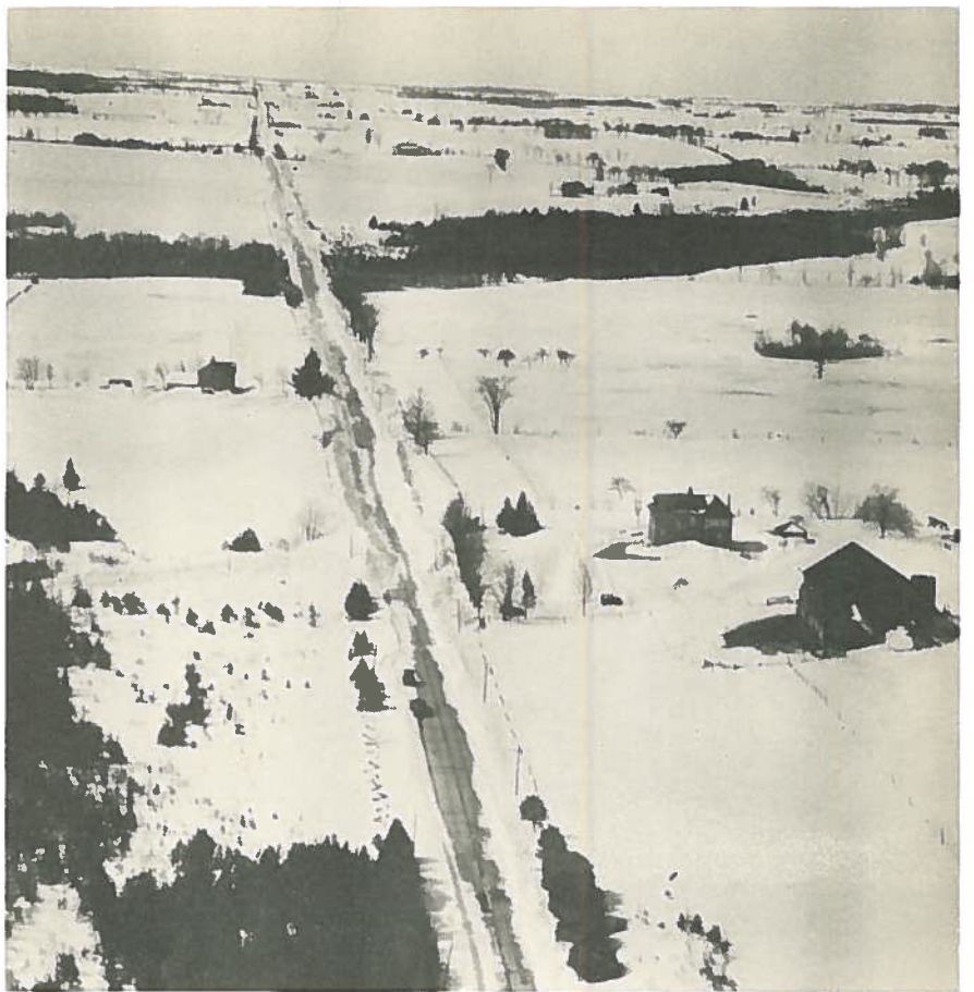
Highway Protected by Woodland: The protection afforded the highway by trees is well illustrated here. Note how the stretches of road sheltered by woodlots are clear of snow whereas huge drifts have formed opposite the open fields.
