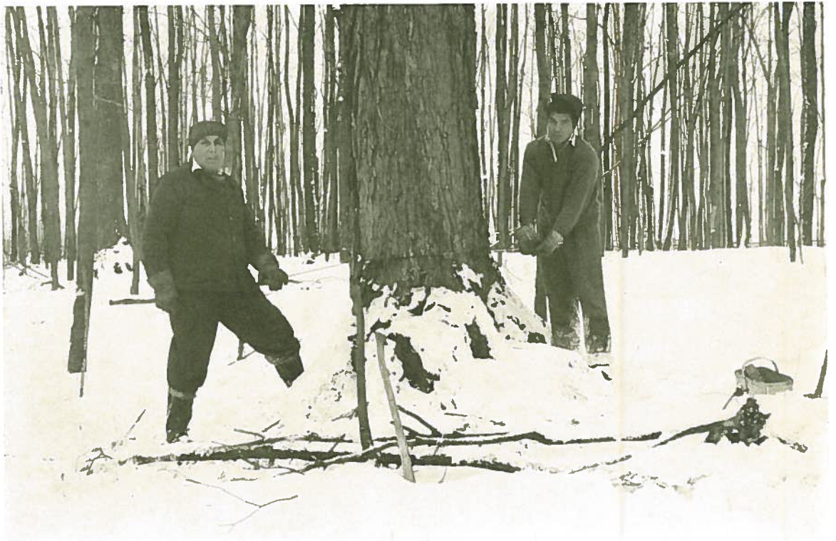
Experienced cross-cut felling gangs can make about 4,000 board feet of hardwood logs (Doyle Rule) per day.
