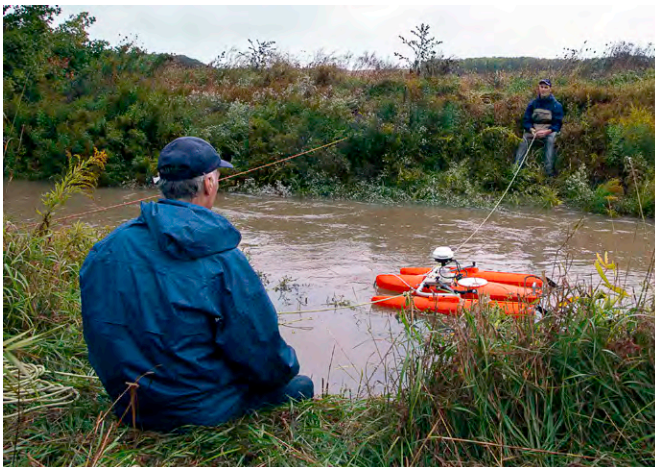
During high flows, the ADCP boat is used to capture flow data when stream levels are too high to safely enter the water.
