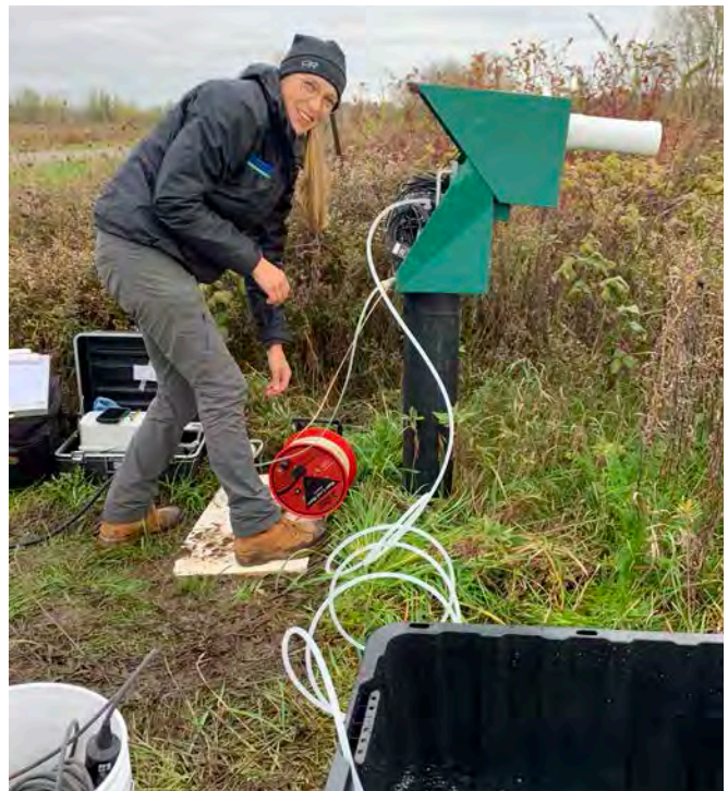
Kaela Orton, Monitoring Technician, takes water samples and collects continuous water level data at a groundwater monitoring well at Golspie Swamp.
