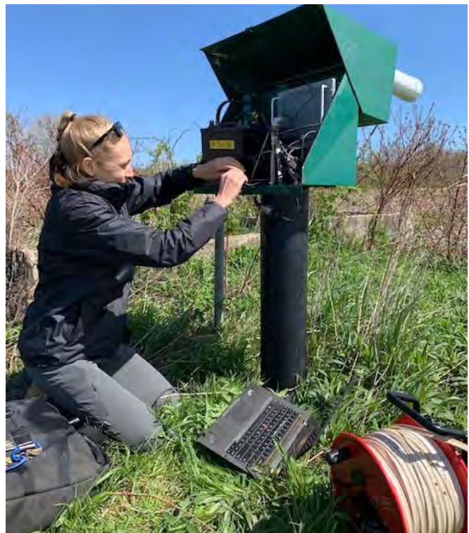
Kaela Orton, Monitoring Technician, downloads groundwater level data at the monitoring well at the Golspie Swamp.
