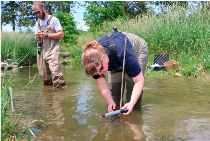
Installing meters for continuous water quality measurements in Medway Creek in-stream restoration site.
