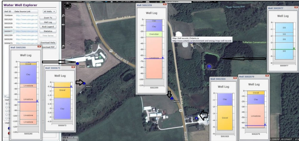
Figure 2: Location of wells in the area and the nature of the aquifers at depth. There are both shallow overburden wells (less than 15 m depth) and deep bedrock wells tapping water between 70 and 120 m depth. The graphic superimposed on the aerial photography is a representation of the materials encountered at depth as described by the well driller. The colour indicates material and the aquifers are represented by gravel and limestone, depth of the well is indicated in meters. ( http://analysis.gw-info.net/gin/publicgin.aspx )
