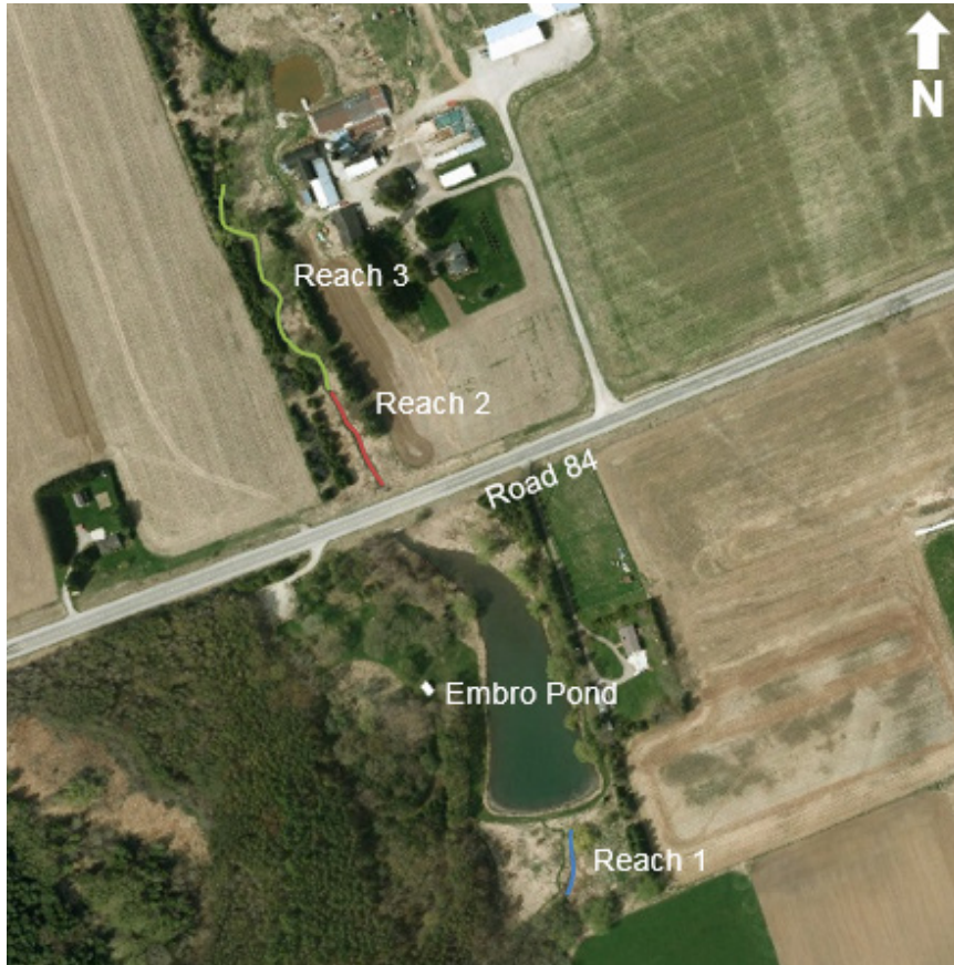
Figure 12 Reach Delineation Along Youngsville Drain
