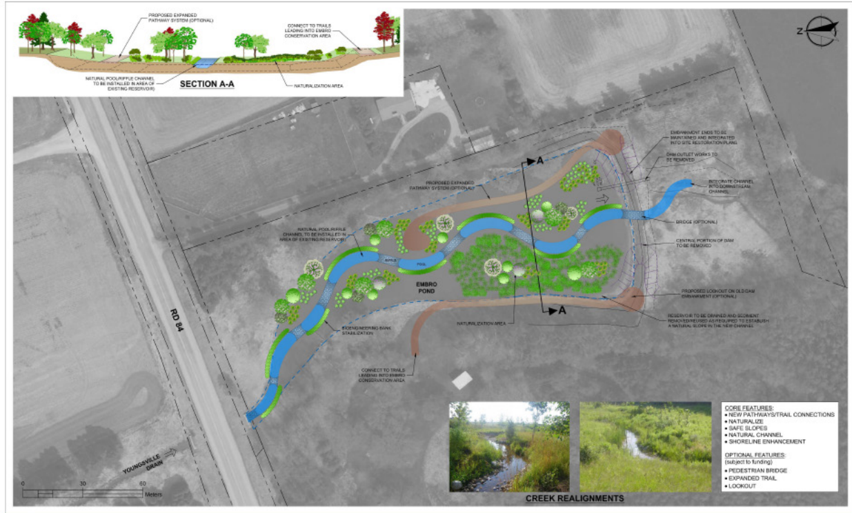
Figure 20 Alternative 3: Remove Dam and Establish Natural Channel
