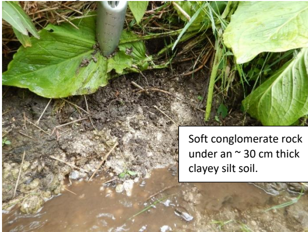
Bank stratigraphy includes a lower unit that provides bedrock control on profile development.
