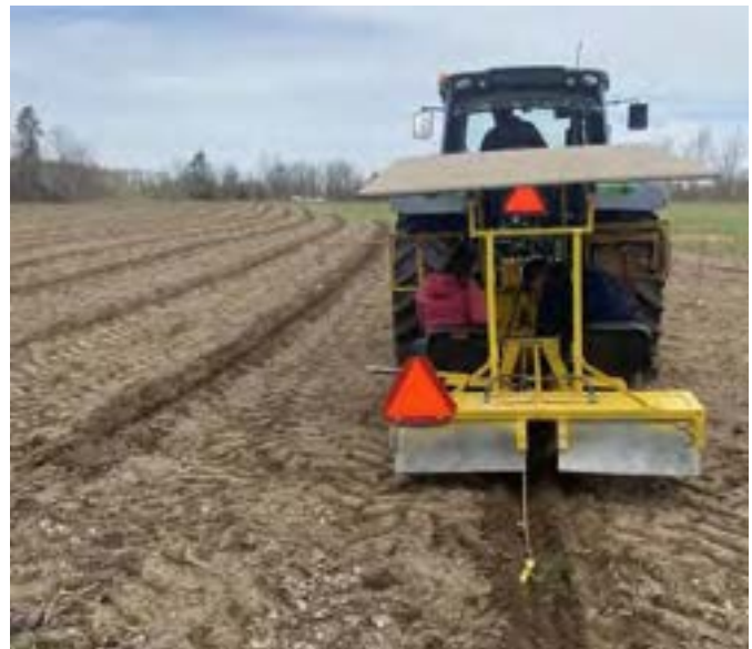
Blocks of trees are planted using a machine planter in a prepared field.
