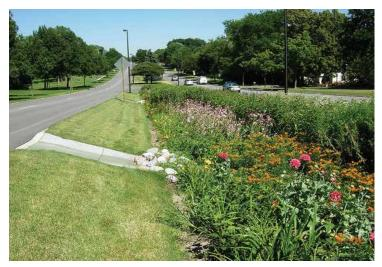
The UTRCA is interested in increasing the implementation of Low Impact Development (LID) in the watershed. LID is a stormwater management technique that uses simple designs and landscape features at the lot level to in infiltrate, filter and retain runoff close to its source. Examples include rain gardens, permeable pavement and bioswales.
