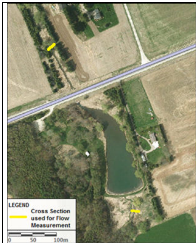
Figure 4: Locations of Cross Sections Used for Stream Flow Measurement at Embro
