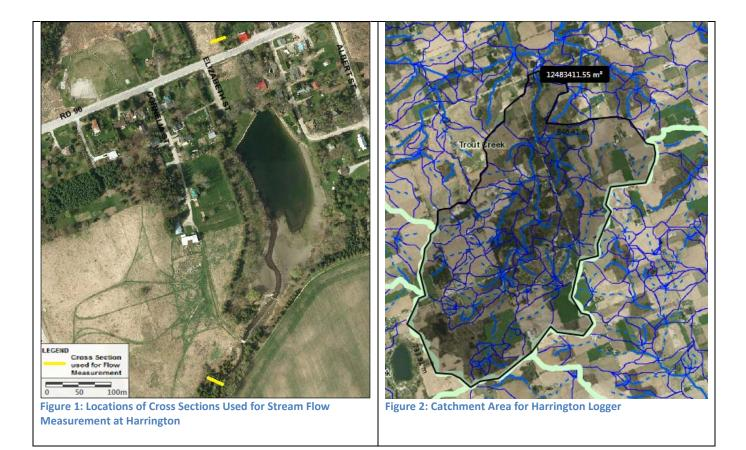
A rating curve was developed to indicate the relationship between the stream flow measured at the most downstream cross section and water level at the Road 96 Bridge Pier; this relationship would allow the conversion of the time series of water level data into a time series of flows. It was determined that there was a logarithmic relationship between the stream flow in liters per second (L/s) and the water level in meters (m).
