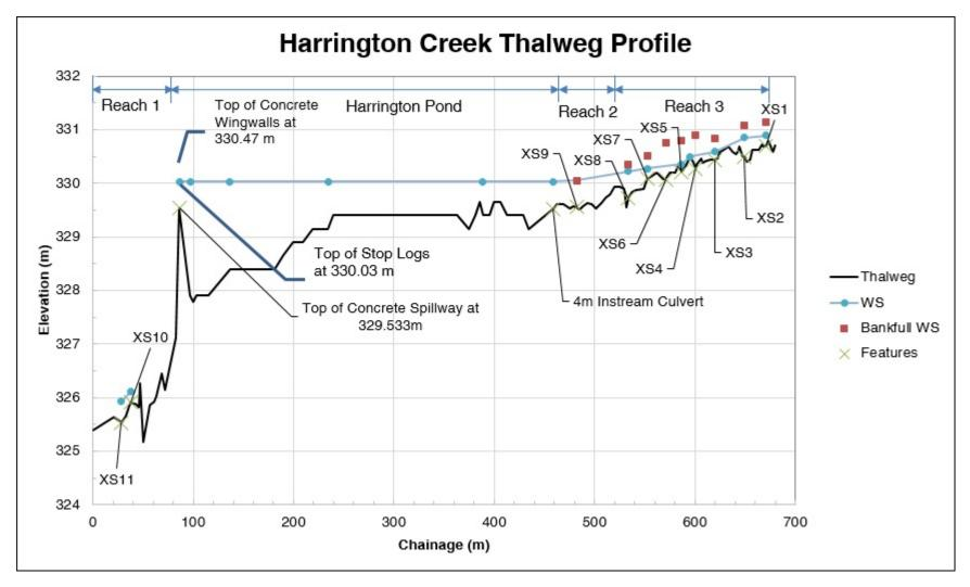
Figure 1-5. Channel bed profile along Harrington Creek
