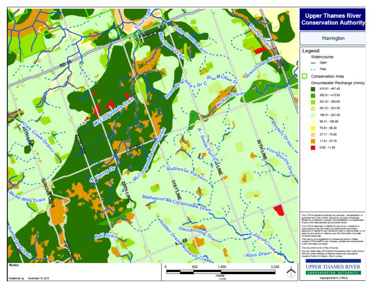
Figure 7: Groundwater recharge (mm/y) of the area around Harrington CA
