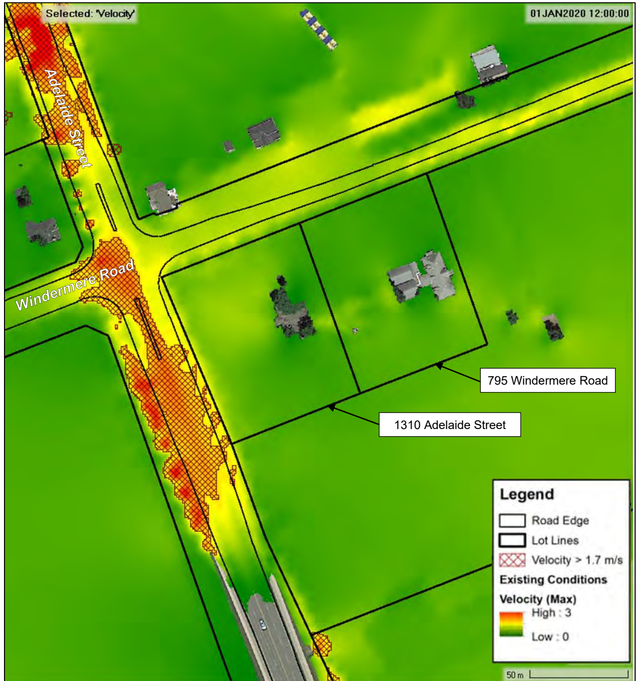
Figure 12: Existing Conditions (BOC Model) Velocity for the Regulatory Flow Event (1250 cms).
