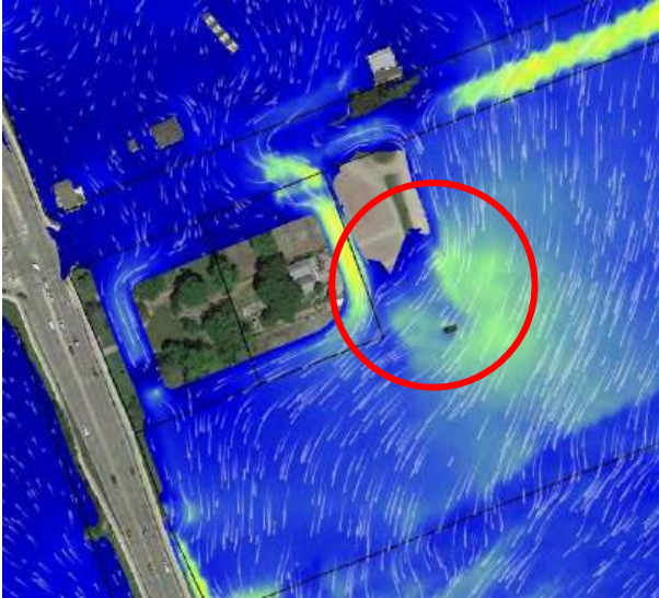
a) 850 cms flow for the partially floodproofed parking lot. Flow moves from north east to south west through the parking lot area (circled in red).
