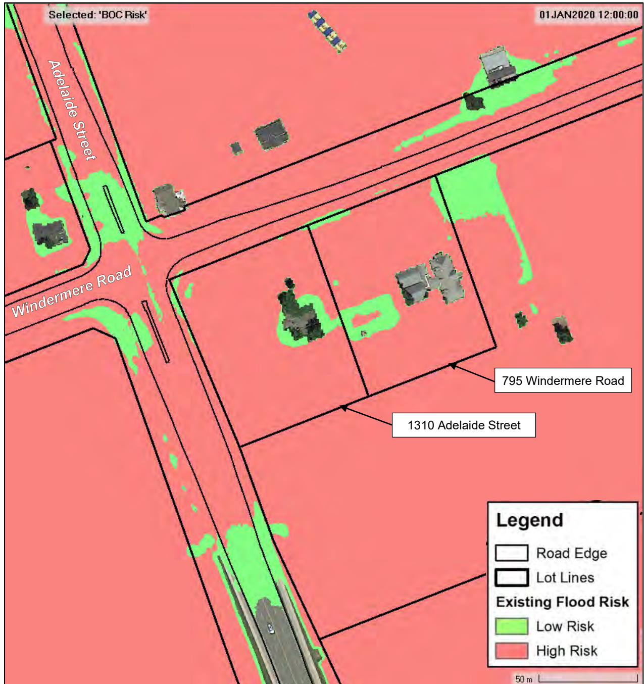
Figure 14: Existing Conditions (BOC Model) Flood Risk for the Regulatory Flow Event (1250 cms).
