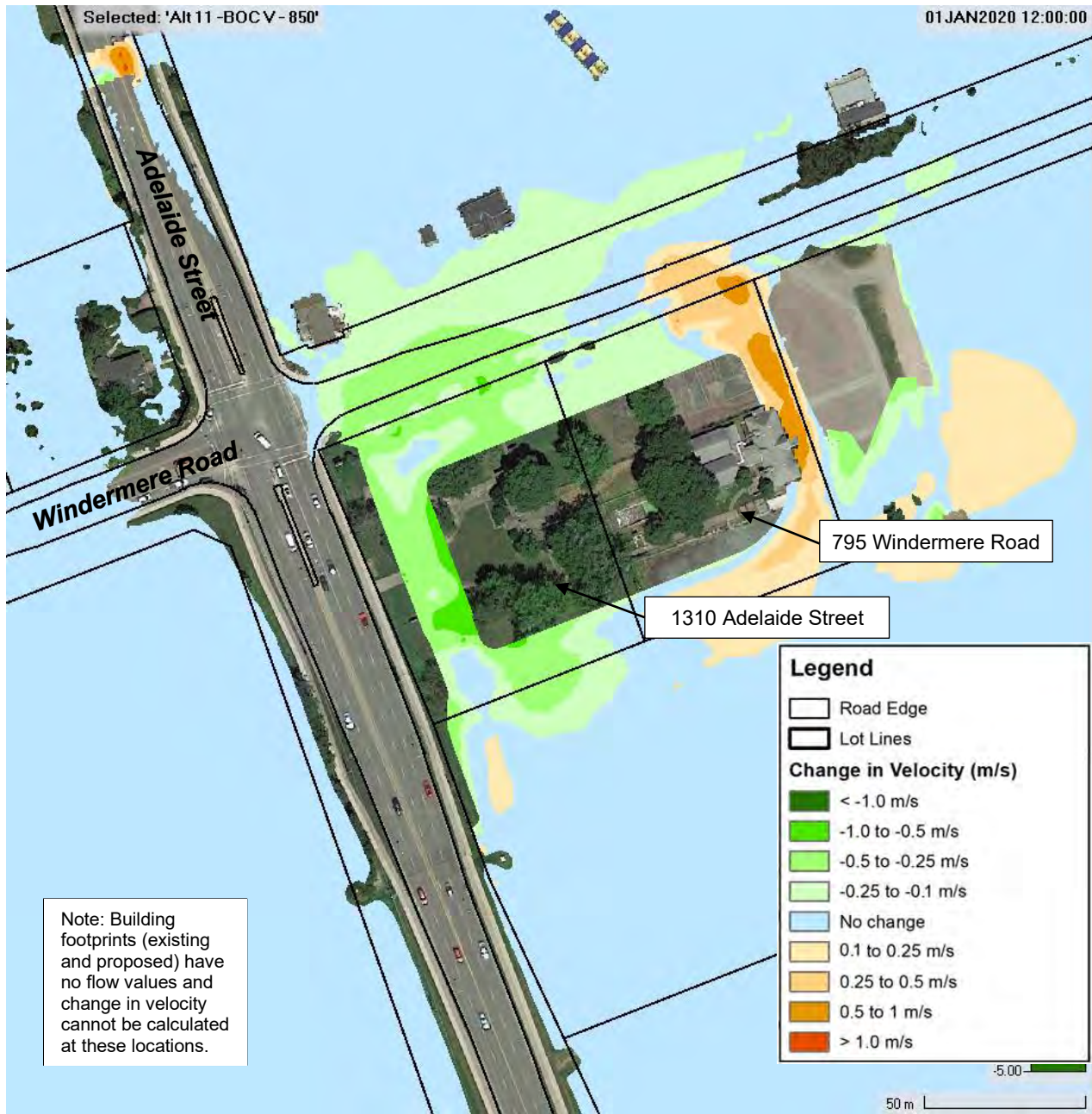
Figure 22: Preferred Site Layout – Change in Flow Velocity for the 850 cms Flow Event
