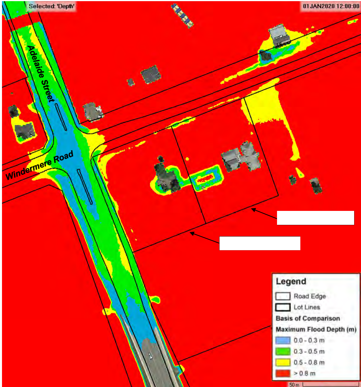
Figure 13: Existing Conditions (BOC Model) Flow Depth for the Regulatory Flow Event (1250 cms).
