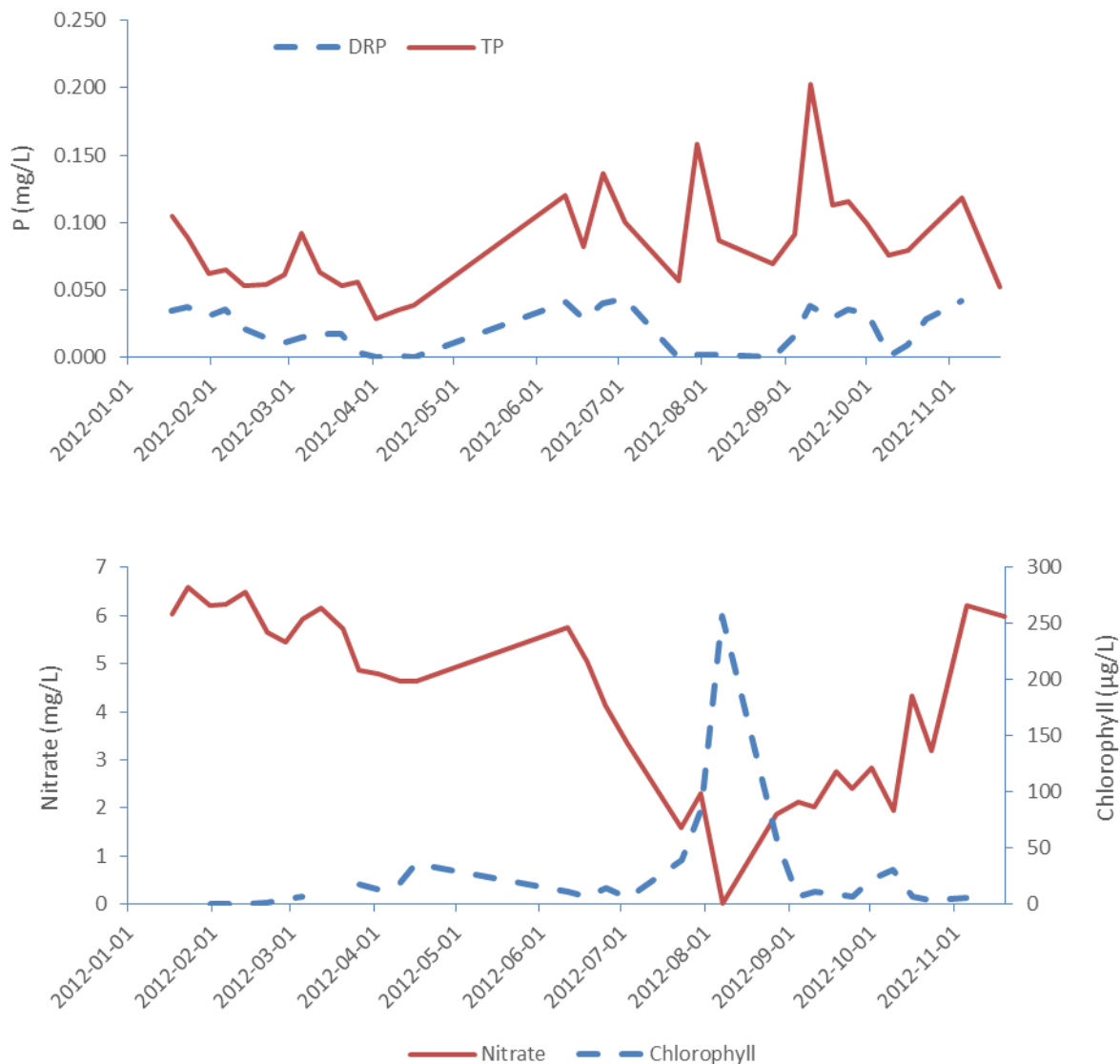
Figure 37 Water quality variables at the frequently sampled EC station 2GE1000 at 65.2km
