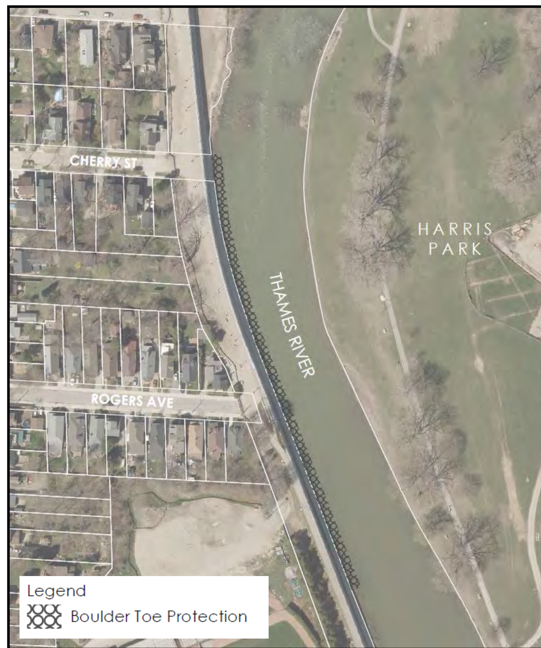
Alternative 1 – Boulder Toe Protection
