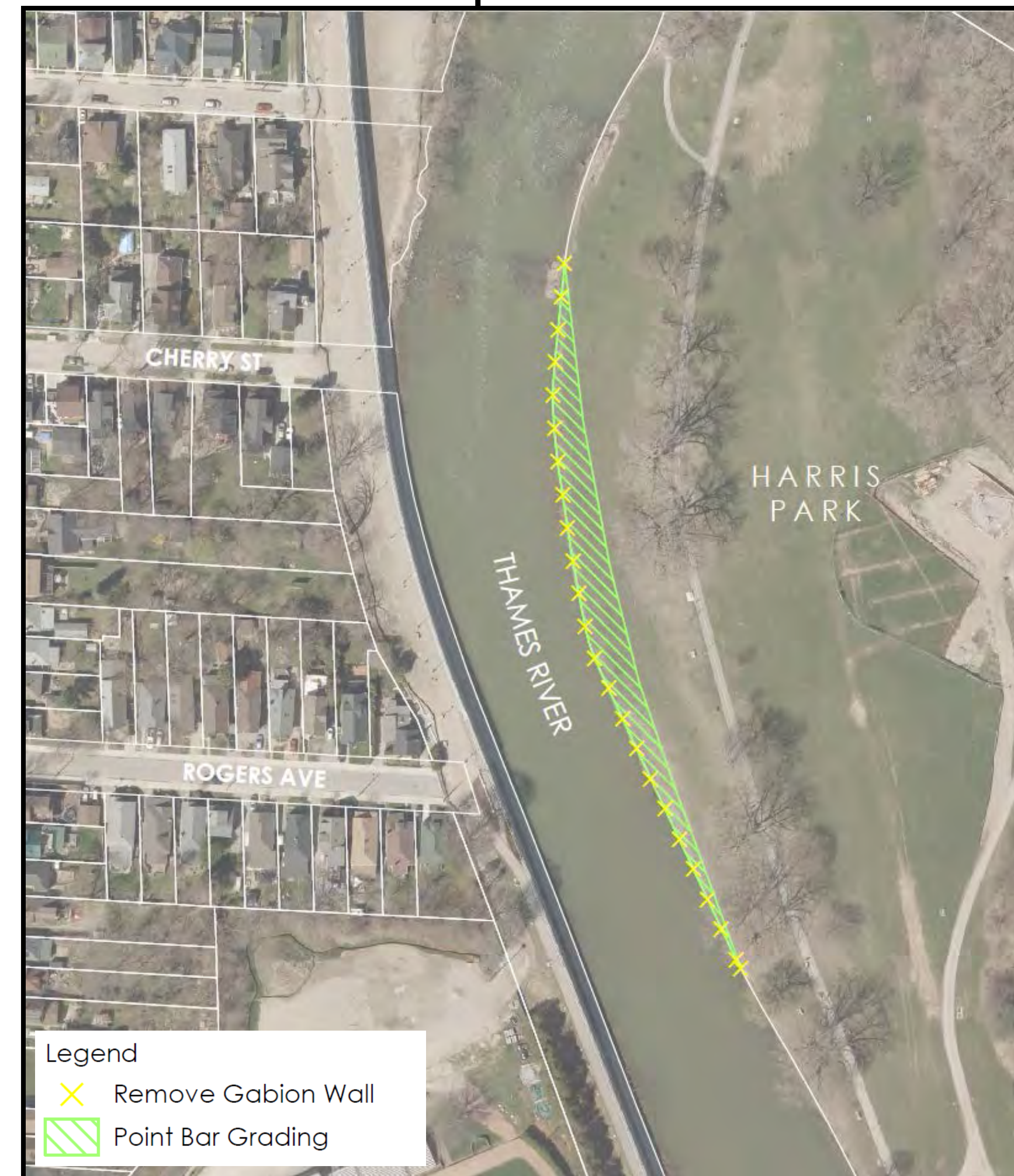
Alternative 2 – Remove Gabions and Reshape Point Bar
