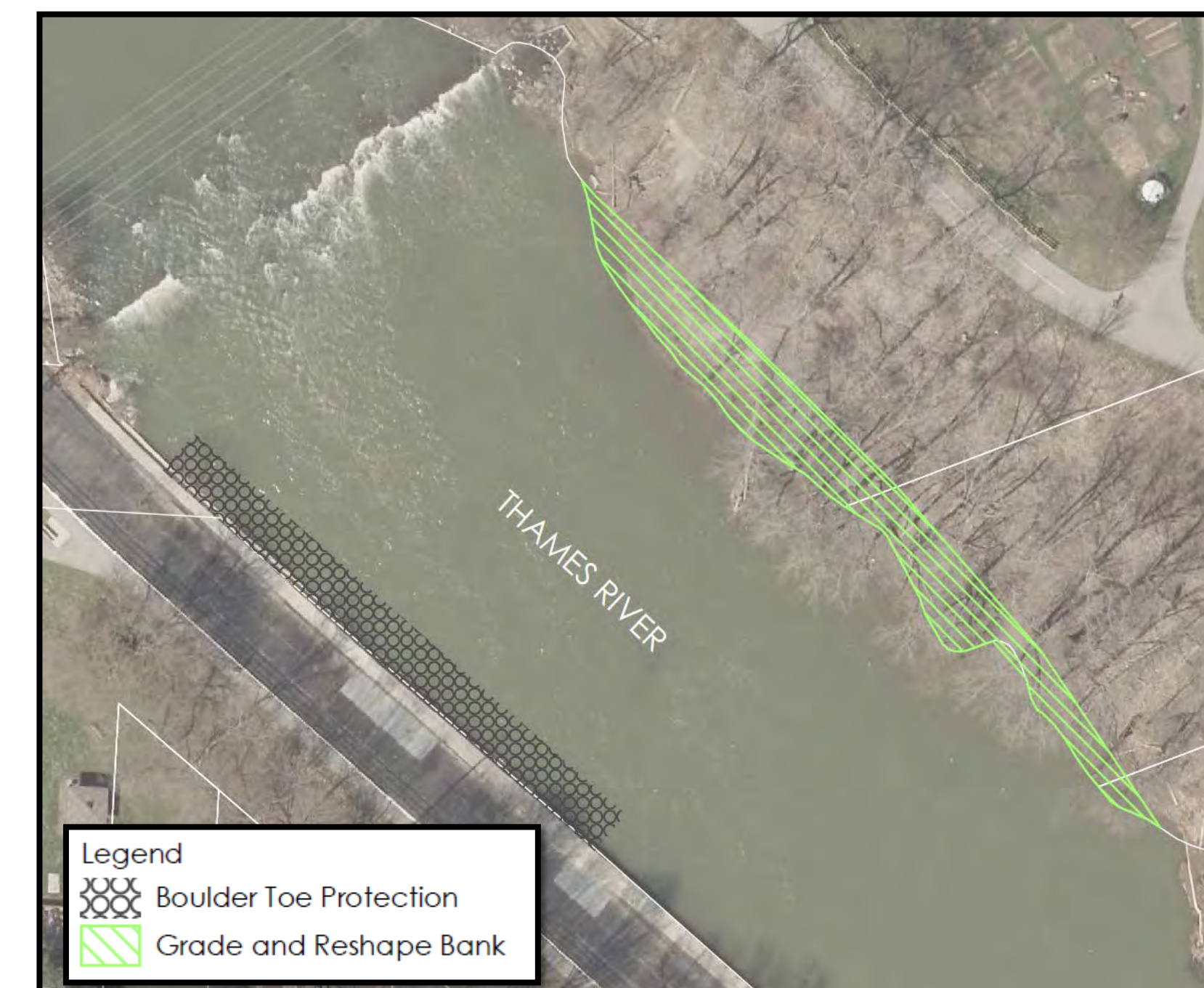
Alternative 3 – Boulder Toe Protection
