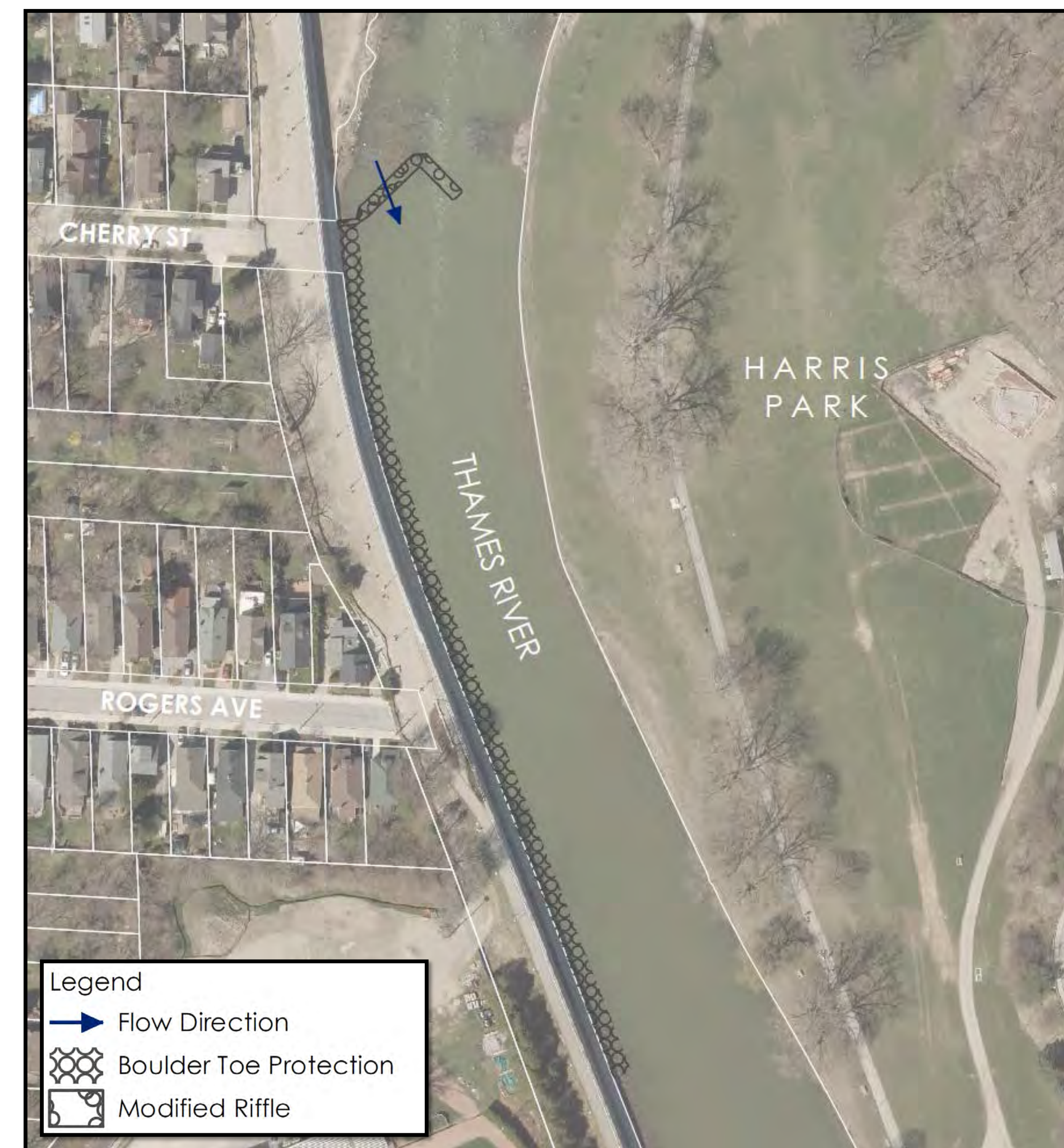
Harris Park Site Modification to MNRF Fish Weirs and Boulder Toe Protection
