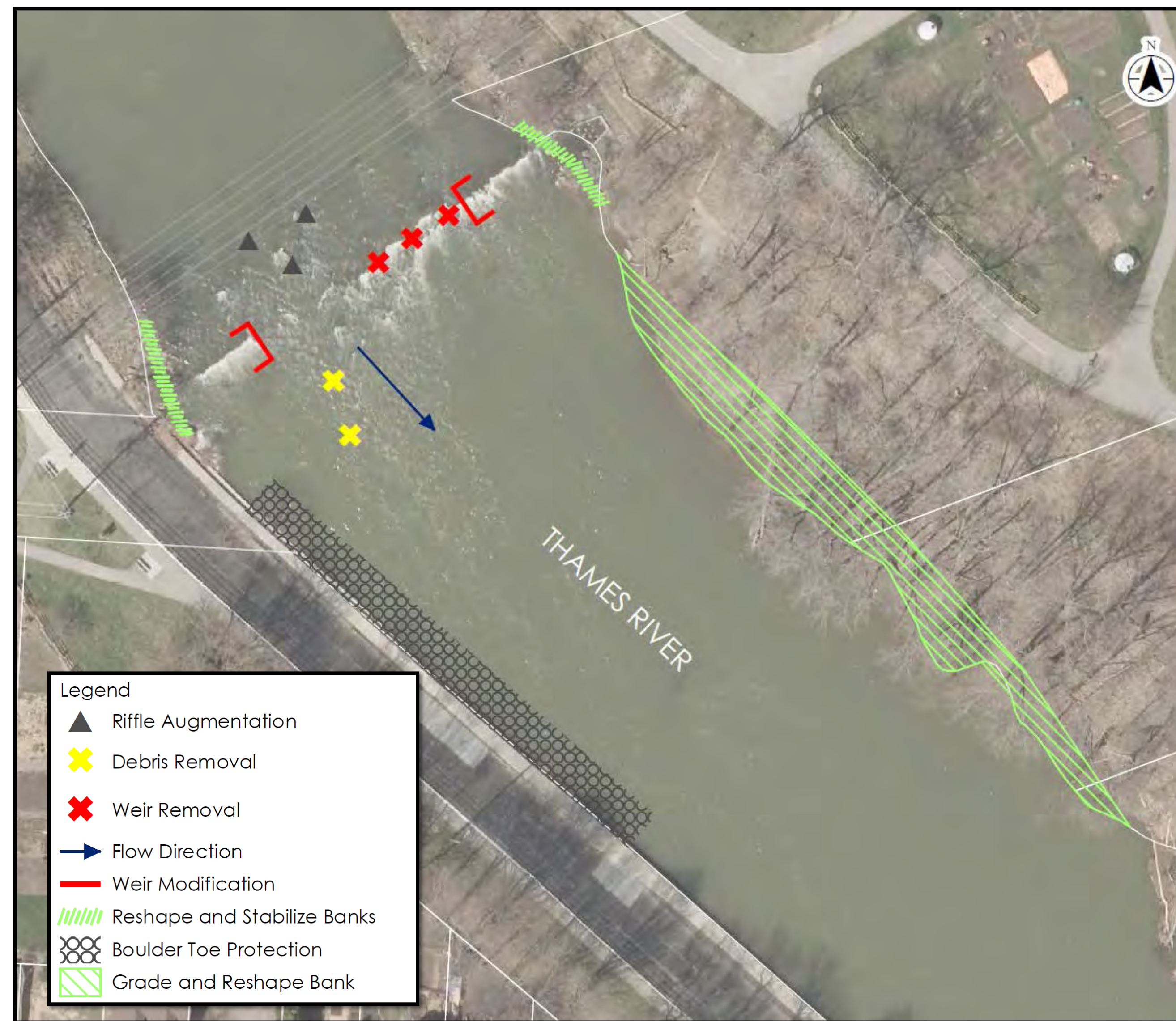
Ann Street Site Modification to Weir Structure and Boulder Toe Protection
