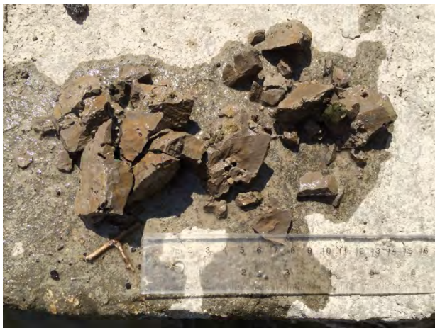
Photo 1-3 – Ann Street Site. Sample of weathered silt till collected from site. The material is friable and easily eroded. Freshly exposed till is resistant to fluvial erosion.
